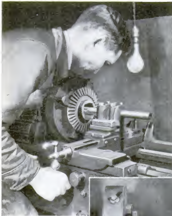
The holder is not only excellent for boring as shown above but also for drilling as at the right, or for reaming, if a suitable sleeve is turned to fit the hole
